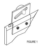
**Note:** Apply a bead of silicone (GE1200) into the open channel of roller bracket (15) before attaching to glass. After placing roller brackets on glass, tighten screw until metal is depressed by 1/32". Allow silicone to cure for 12 hours before hanging panels.
